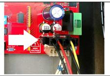
**Step 3: Power Harness Installation** Find the power harness from the accessories box and connect the black connector to the motor board as shown in the above photo.
