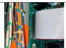
Step 5b: Ribbon Cable Installation
