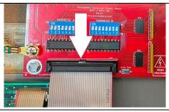
Step 5c: Ribbon Cable Installation
