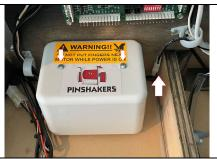
**Step 7h: Shaker Motor Installation** Install the shaker motor plastic shield with the two small shield screws and plug in the motor to the motor harness.
