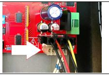
Above shows where you connect the wire harness you removed from the power driver board if both connections there were occupied. The 20vac / 50vac output on the motor board is just a pass-through connection. The voltages are not altered in any way so it will not have any affect on your machine's components.
