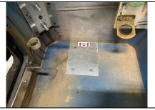
Step 7b: Shaker Motor Installation Included is a metal drill guide with 4 predrilled holes that you will use to drill the 17/64" holes in the cabinet. Place the drill guide against the side wall in the spot you believe you want the motor to be mounted.
