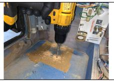
Step 7e: Shaker Motor Installation Drill your 4 holes using the included 17/64" drill bit. It is VERY important to keep your drill completely perpendicular to the bottom of the cabinet. If you make your drill holes at any kind of an angle, then the tee nuts will not fit properly and your motor will not install securely. Take your time and be patient, you only get one shot at this!
