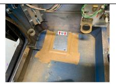
**Step 7d: Shaker Motor Installation**Tape the drill guide in place so that it will not move.
