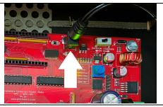
Step 6a: Motor Harness Installation Grab the motor harness out of the accessories box and connect the barrel plug into the motor driver board. Run the cable down the side of the backbox and into the back of the cabinet.
