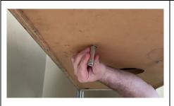
Step 7f: Shaker Motor Installation Once you get all 4 screws drilled, go underneath and hammer in the 4 tee nuts. Use a 1/2" deep socket to help so you don't smash your fingers. Hammer the tee nuts as far in the cabinet as they will go. If they do not go all the way in they will finish flush when you screw in the hex screws in the next step.
