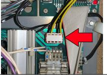
Step 4: Power Harness Installation Connect the power harness to the machine's power driver board. For WPC era machines use either J104 or J105. For WPC-95 machines use either J130 or J131. The connectors are all the same.
