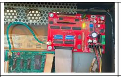
Step 1: Motor Driver Board Install Find an open spot in the upper right side of the backbox to secure the motor board with the four 1" hex head wood screws in the hardware bag. If able try to line up the top left screw to go through one of the metal grill holes first.
