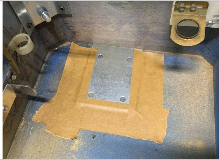
**Step 4:** Tape the drill guide in place so that it will not move.
