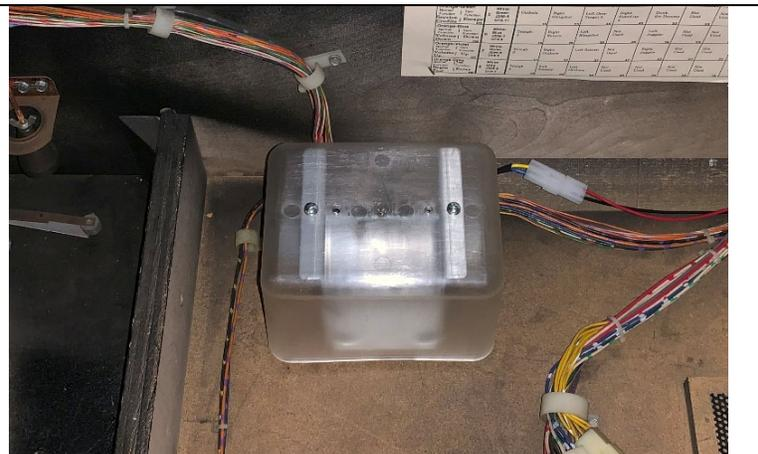
To the right is an example of the motor installed on the raised transformer deck. For this you will use the included 2" mounting screws.
