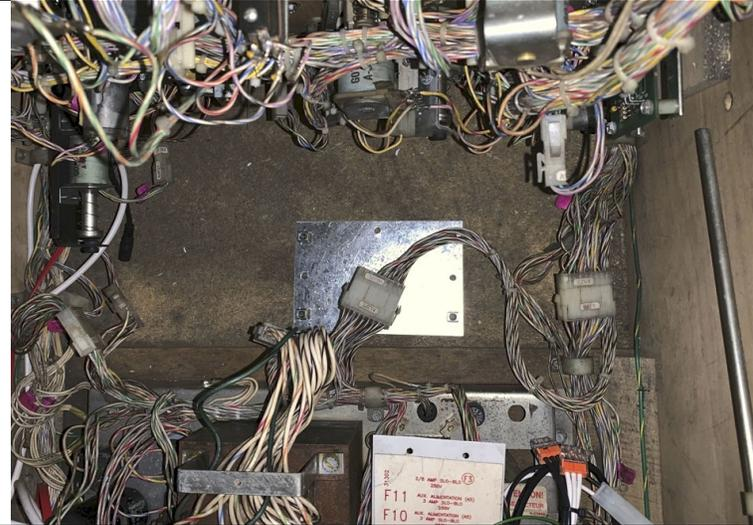
You received a metal Backplate with your kit that is used to mount the motor driver board. The picture to the right shows the spot in the cabinet where you will secure it with the 4 hex head wood screws in the hardware bag.
