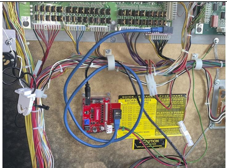
To the right is an example of where you can install the board in the older Whitestar generation machine using just the velcro.. This photo was taken with the an older version motor board, but it should still give you a good idea of where you can mount it.
