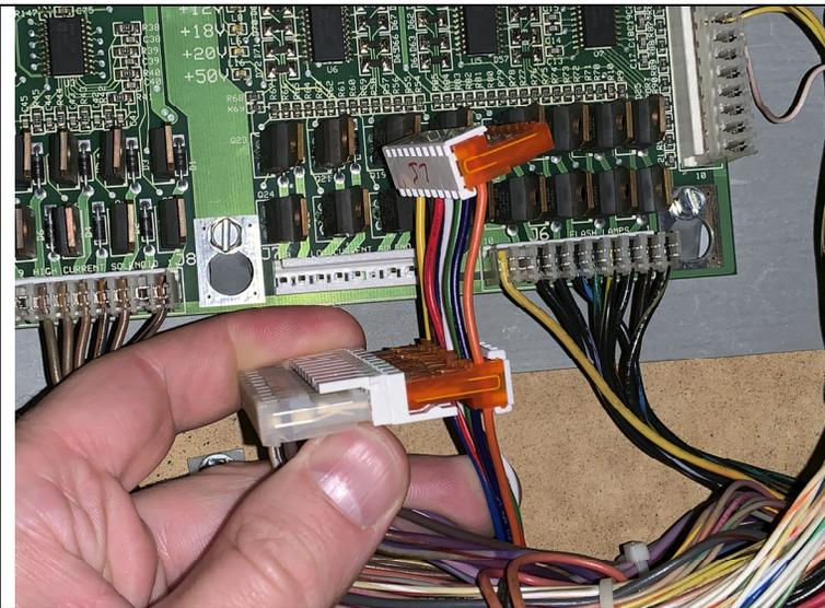
**Step 6:** Locate the power driver board connector for the type of wire harness you have. Unplug it and connect it inline with the “Z” adapter on the wiring harness. It will come pre-keyed and pre-labeled. Here is a quick reference list:
