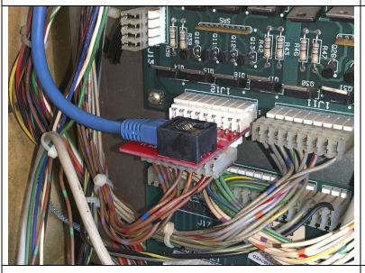
**Step 6:** Locate the power driver board connector for the type of machine you have. Unplug it and connect it to the connection on the bottom of the Cat5 adapter. Then connect the adapter back into the power driver board. Last, connect the Cat5 cable to the adapter. A photo to the left is a side view of the "A" adapter at 1J12.
