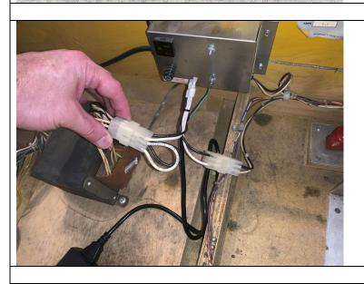
Separate the 9pin jumper connector from the connector coming out of the transformer. There is a small tab you will have to lift up on one of the side in order to separate the two connectors. Insert the pre-jumpered end of the included adapter into the transformer connector. Then insert the connector coming from your power box into the other side of the included adapter. When you are all finished, the connection should look like the photo to the left.
