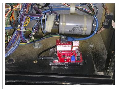
To the right is an example of an alternate location for the motor driver board. You can use one of the holes predrilled in the metal back plate to mount one side of the driver board case, and also use the velcro to ensure a secure fit.
