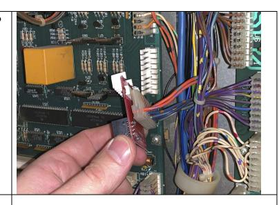
\*\*\*Whirlwind Only\*\*\* - Whirlwind has a special additional circuit board called a "Sound Overlay Solenoid Board". It is located to the left of the power supply. There is no harness "A" for a Whirlwind, instead there is a harness "C" which will connect to J4 of this Aux board. Look at the photo to the right of reference. The harness adapter you will use will be the standard Sys11 harness "A" adapter, however there will be two extra pins that are not connected.
