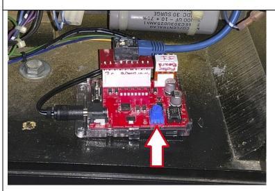
**Step 9:** Power the machine on and look for the led on the motor driver board. It should flash 5 times during it's power-on routine. Once it is steady green, it is ready for action. Press the test button next to the fuse and the motor should shake. If it doesn't, then go back through the above steps to make sure you didn't miss a connection somewhere.
