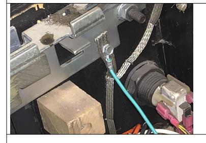
**Step 2:** Take the 1/4" nut driver and install the grounding cable to the grounding braid as shown in the image to the left. This is very important!
