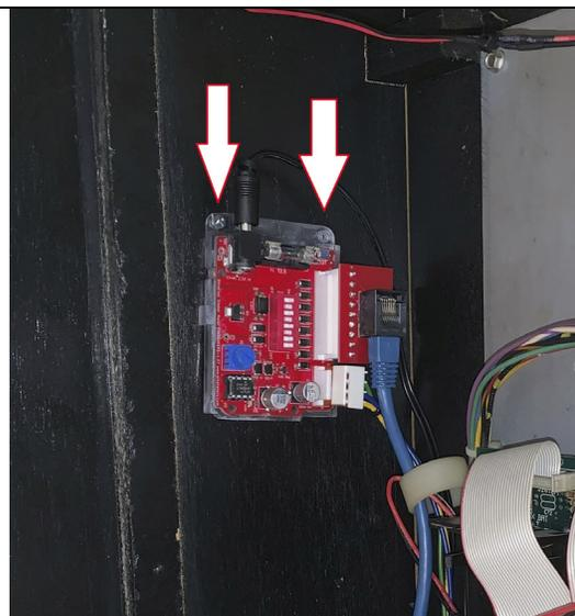
**Step 10:** Use the two wood screws to secure the driver board to the side of the backbox. Only use the two mounting holes at the top of the case as shown in the picture to the left. Do not use any of the other holes that are on the driver board.
