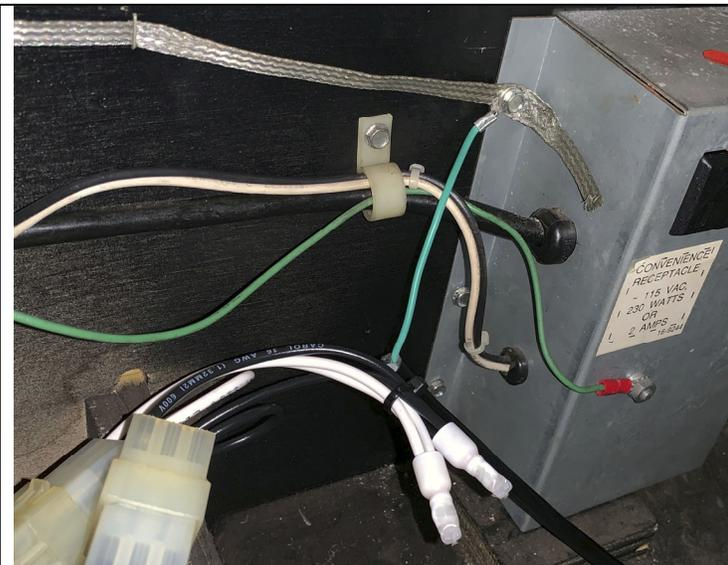
**Step 6:** Connect the grounding wire to the machine. I prefer to use the 1/4" nut drive screw that is used to secure the grounding braid. You can also connect it to the 11/32" nut that is securing the grounding cable on the side of the power box.
