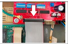
**Step 5c: Ribbon Cable Installation** Connect the other end of the ribbon cable to the motor driver board. The red stripe should be positioned on the right side.
