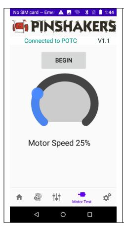
**Step 14: Motor Test** You can test the motor within the app to make sure it is working and everything is installed properly. You can also use the motor test function to get an idea of how strong you want the motor to be.
