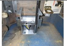
**Step 7f: Shaker Motor Installation** Once you get all 4 screws drilled, go underneath and hammer in the 4 tee nuts. Use a 1/2" deep socket to help so you don't smash your fingers. Hammer the tee nuts as far in the cabinet as they will go. If they do not go all the way in they will finish flush when you screw in the hex screws in the next step.
