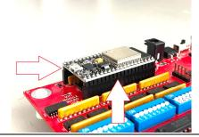
**Step 8b: Premium Upgrade** Take the premium upgrade module and line up the pins with the header on the motor driver board. Make sure the micro USB connector is facing on the left side as shown in the above image. Push the module into the header and make sure it is all the way down and that all of the pins are aligned properly.
