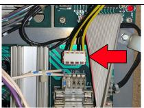
**Step 4: Power Harness Installation** Connect the power harness to the machine's power driver board. For WPC era machines use either J104 or J105. For WPC-95 machines use either J130 or J131. The connectors are all the same. If there are no open connections, remove one of them and plug that connector into the 20vac / 50vac output connection on the motor driver board. After that, connect the power harness to the connection you just freed up on the power driver board.
