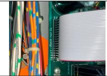
**Step 5b: Ribbon Cable Installation** Be very careful when installing the new ribbon cable as it is possible for the connection to be miss-aligned. The above photo is an example of the connection installed with only half of the pins connected. Make sure you have plenty of light and do not try to force the plug in as that is a good sign it is not aligned correctly.
