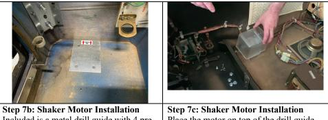
Step 7b: Shaker Motor InstallationSIncluded is a metal drill guide with 4 pre-<br/>drilled holes that you will use to drill the<br/>17/64" holes in the cabinet. Place the<br/>drill guide against the side wall in the<br/>spot you believe you want the motor to be<br/>mounted.S
