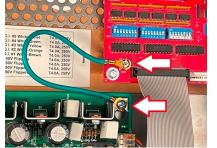
Step 2: Grounding Strap Installation Find a reliable grounding source. You can secure it to the backbox metal panel, a part of the grounding strap, or connect it to one of the board mounting screws like the photo above. Installing this kit in a machine where something is not properly grounded will result in damage to components. DO NOT SKIP THIS STEP!
