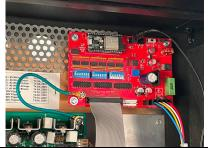
**Step 1: Motor Driver Board Install** Find an open spot in the upper right side of the backbox to secure the motor board with the four 1" hex head wood screws in the hardware bag. If able try to line up the top left screw to go through one of the metal grill holes first.
