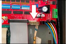
Above shows where you connect the wire harness you removed from the power driver board if both connections there were occupied. The 20vac / 50vac output on the motor board is just a pass-through connection. The voltages are not altered in any way so it will not have any affect on your machine's components.
