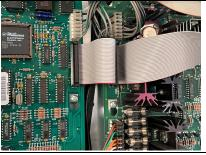
**Step 5a: Ribbon Cable Installation** Locate the ribbon cable in the accessories box. We will be replacing the short ribbon cable that is connected between the MPU and the Power Driver Board. Carefully remove the original ribbon cable and be sure not to bend the little pins. Replace it with one provided with the kit. The photo above shows how you need to orient the cable. Make sure the red stripe is on the bottom.
