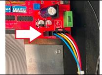
**Step 3: Power Harness Installation** Find the power harness from the accessories box and connect the black connector to the motor board as shown in the above photo.
