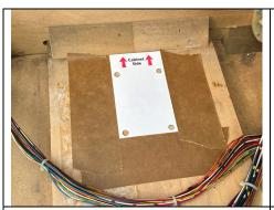
**Step 7d: Shaker Motor Installation**Tape the drill guide in place so that it will not move.
