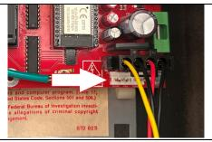
Above shows where you connect the wire harness you removed from the power driver board if both connections there were occupied. The connector is labeled "J4" on the motor board. The 20vac / 70vac output on the motor board is just a pass-through connection. The voltages are not altered in any way so it will not have any affect on your machine's components.
