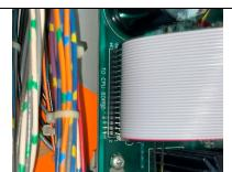
Step 5b: Ribbon Cable Installation
