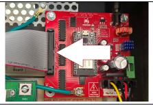
**Step 5c: Ribbon Cable Installation**Connect the other end of the ribbon cable to the motor driver board. The red stripe should be positioned on the bottom like the picture above.
