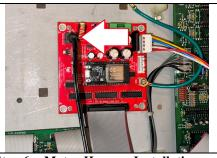
Step 6a: Motor Harness Installation
