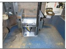
Step 7g: Shaker Motor Installation
