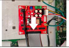
**Step 5c: Ribbon Cable Installation**Connect the other end of the ribbon cable to the motor driver board. The red stripe should be positioned to the right like the picture above.
