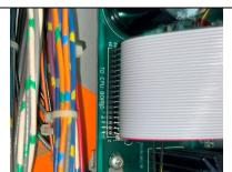
Step 5b: Ribbon Cable Installation
