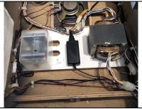
Above is an example of the motor installed on the raised transformer deck. For this you will use the included 2" mounting screws. Be careful how tight you screw the bolts in as there is an open gap under this transformer deck and you don't want to snap the wood as you are tightening them.
