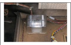
Step 7a: Shaker Motor Installation Choose where you would like to install your shaker motor. We have discovered you get the best results by installing the motor as close to the side and front of the cabinet as possible. If you can't fit the motor in the front compartment, then place it on the other side of the divider into the middle section.
