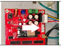
Above shows where you connect the wire harness you removed from the power driver board if both connections there were occupied. The connector is labeled "Aux" on the motor board. The 20vac / 70vac output on the motor board is just a pass-through connection. The voltages are not altered in any way so it will not have any affect on your machine's components.
