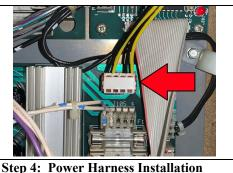
Connect the other side of the power harness to the machine's power driver board. WPC era machines use either J104 or J105. WPC-95 machines use either J130 or J131. They are the same. You may need to remove one of them and plug that connector into the "Aux" connection on the motor driver board. After that, connect the power harness to the connection you just freed up on the power driver board.
