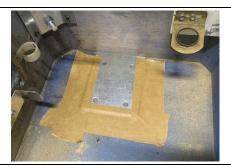
**Step 6c: Shaker Motor Installation** Tape the drill guide in place so that it will not move.
