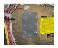
Step 1: Motor Driver Backplate Install Find an open spot in the backbox to secure the backplate with the 4 hex head wood screws in the hardware bag. It is OK if the plate is mounted over a grounding strap or grill. Whitestar machines may require the plate to be installed on one of the sides inside the backbox.
