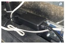
Step 4a: Power Supply Installation
