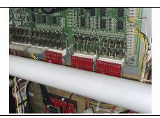
**Step 3a: Harness Adapter Installation** Replace the lamp if you removed it. The photo above shows the adapters installed with the lamp in place.
