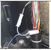
Step 4: Power Supply Installation Find the 2 position molex connection leading to the backbox lamp. It is usually on the left side of the backbox coming up from the back of the cabinet. Disconnect the molex connection and connect the included power supply cable "Y" adapter into it.
