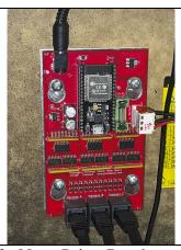
Step 2: Motor Driver Board Installation
