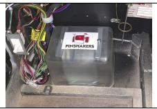
**Step 6g: Shaker Motor Installation** Install the shaker motor plastic shield with the two small shield screws and plug in the motor to the motor harness.
