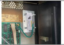
Step 1: Motor Driver Backplate Install Find an open spot in the upper right side of the backbox to secure the backplate with the 4 hex head wood screws in the hardware bag. It is OK if the plate is mounted over a grounding strap or grill.
