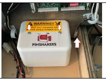
**Step 7g: Shaker Motor Installation** Install the shaker motor plastic shield with the two small shield screws and plug in the motor to the motor harness.
