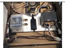
Above is an example of the motor installed on the raised transformer deck. For this you will use the included 2" mounting screws.
