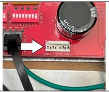
Above shows where you connect the wire harness you removed from the power driver board if both connections there were occupied. The 20vac / 50vac output on the motor board is just a pass-through connection. The voltages are not altered in any way so it will not have any affect on your machine's components.
