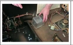
Step 7b: Shaker Motor Installation
