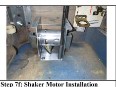
Use a drill, 5/16" socket, and an extension to drill in the screws and compress the tee nuts the rest of the way flush with the cabinet. Reach under with one hand and hold the tee nuts from falling out during this step. It is best not to tighten down
