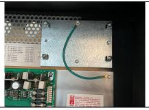
**Step 1: Motor Driver Backplate Install** Find an open spot in the upper right side of the backbox to secure the backplate with the 4 hex head wood screws in the hardware bag. It is OK if the plate is mounted over a grounding strap or grill.
