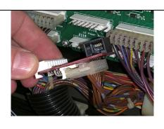
Step 5: Harness Adapter Installation Locate the power driver board connector for the type of machine you have. Printed on each Cat5 adapter is the harness identifier as well as the Jxxx connection on the power driver board. Unplug the connector on the power driver board and connect it to the bottom of the Cat5 adapter. Then connect the adapter back into the power driver board.
