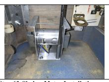
Step 6f: Shaker Motor Installation
