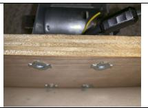
Here is an example of properly installed tee nuts. See how they rest flush with the wood. If your tee nut falls out while you are trying to screw them in, that means you probably did not hammer them in far enough. Make sure you take a pair of pliers and straighten out the prongs before you try to re-install it.
