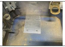
Step 6a: Shaker Motor Installation Included is a metal drill guide with 4 predrilled holes that you will use to drill the 1/4" holes in the cabinet. Place the drill guide against the side wall in the spot you believe you want the motor to be mounted.
