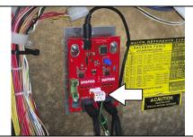
**Step 5: Motor Harness Installation**Connect the motor harness into the motor board as shown in the photo above.
