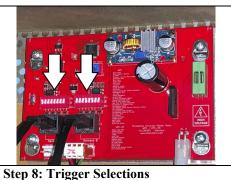
Feel free to change the dip switch settings with a pen or other like device on the motor driver board for the desired inputs that you want to drive the shaker motor. Do this while the machine is powered down. You can choose to have more than
