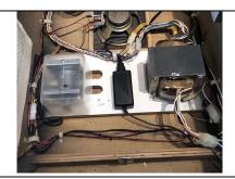
Above is an example of the motor installed on the raised transformer deck. For this you will use the included 2" mounting screws.
