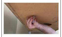
Step 7e: Shaker Motor Installation Once you get all 4 screws drilled, go underneath and hammer in the 4 tee nuts. Use a 1/2" deep socket to help so you don't smash your fingers. Hammer the tee nuts as far in the cabinet as they will go. If they do not go all the way in they will finish flush when you screw in the hex screws in the next step.
