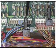
The photo above shows the connections on a WPC-95 machine. Notice how for the Harness "A" it requires that you carefully route the wires coming off of the J111 connector above it. You may even need to remove the J111 connector prior to installing the J112 adapter in order for everything to fit easily.
