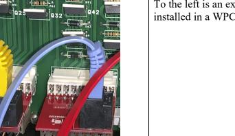
To the left is an example of harnesses "A" & "B" installed in a WPC-95 era machine.
