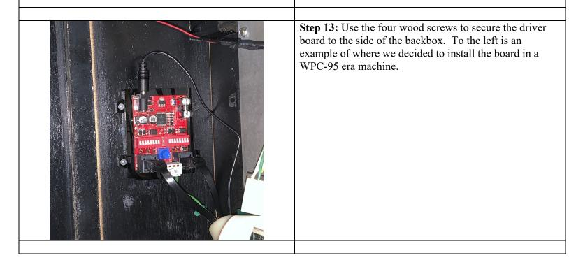
Here is the driver board location for WPC generation machines. This is the older version board but still gives you an idea of where to place the new one. Make sure you keep enough room for the 12vdc connector to easily connect to the driver board. Also make sure you have room for the Cat5 connector adapters.
