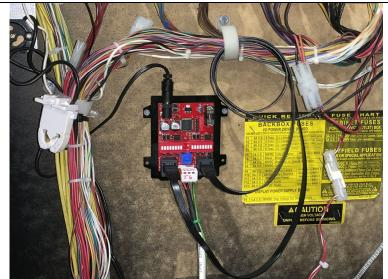
Here is the motor driver board installed in a Stern S.A.M. era machine.
