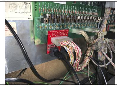
Here is another example of the harness adapter installed to the A3P6 connection.
