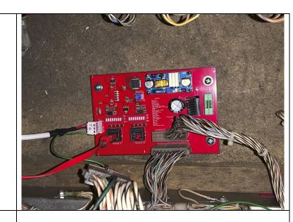
**Step 2b: Motor Driver Board Installation**
