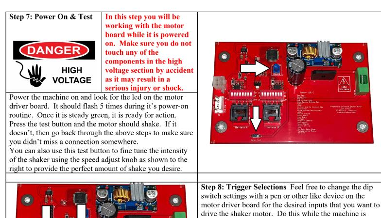
Country settings only. You may turn on any dip switch on the motor driver board that does not have the "Not Used" or "Do Not Use" label on the dip switch chart. You can choose to have more than one switch turned on at a time. Have fun with it and try to make it so that it feels as if this kit was always meant to be installed from the factory.
