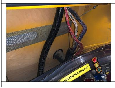
**Step 6: Motor Harness Installation** Now run the motor harness down into the cabinet. Use the wire wraps like the ones shown to the left to neatly secure the wires. Connect the motor harness to the shaker motor, and leave all slack in the lines in the back of the cabinet at the base of these wire wraps. That way when you go to fold the backbox down, the slack will be used and nothing will get caught and ripped out.
