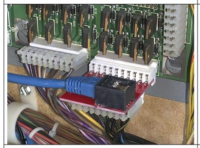
**Step 6:** Locate the power driver board connector for the type of machine you have. Unplug it and connect it to the connection on the bottom of the Cat5 adapter. Then connect the adapter back into the power driver board. Last, connect the Cat5 cable to the adapter. A photo to the left is a side view of the adapter.
