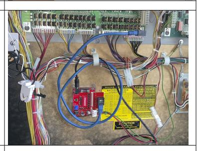
To the right is an example of where you can install the board in the older Whitestar generation machine using just the velcro.. This photo was taken with the an older version motor board, but it should still give you a good idea of where you can mount it.
