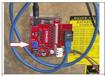
**Step 9:** Power the machine on and look for the led on the motor driver board. It should flash 5 times during it's power-on routine. Once it is steady green, it is ready for action. Press the test button next to the fuse and the motor should shake. If it doesn't, then go back through the above steps to make sure you didn't miss a connection somewhere.
