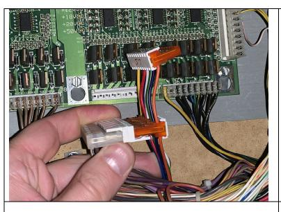
**Step 6:** Locate the power driver board connector for the type of wire harness you have. Unplug it and connect it inline with the "Z" adapter on the wiring harness. It will come pre-keyed and pre-labled. Here is a quick reference list:
