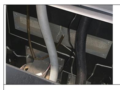
**Step 14:** Now run the shaker motor connection wires down into the cabinet. Use the wire wraps like the ones shown to the left to neatly secure the shaker motor wires. Connect the shaker motor and the power supply, and leave all slack in the lines for both the shaker motor wires and the 12vdc cord in the back of the cabinet at the base of these wire wraps. That way when you go to fold the backbox down, the slack will be used and nothing will get caught and ripped out.
