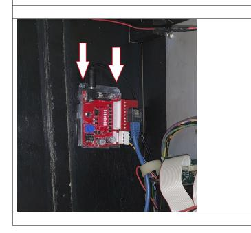
**Step 10:** Use the two wood screws to secure the driver board to the side of the backbox. Only use the two mounting holes at the top of the case as shown in the picture to the left. Do not use any of the other holes that are on the driver board.
