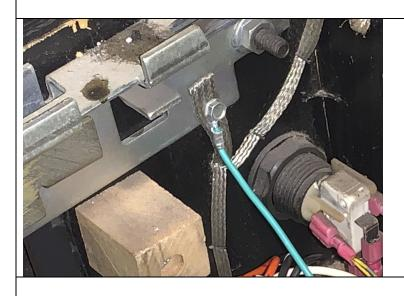
**Step 2:** Take the 1/4" nut driver and install the grounding cable to the grounding braid as shown in the image to the left. This is very important!
