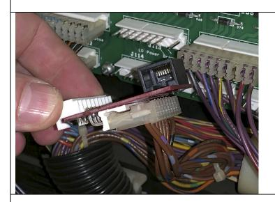
**Step 11:** Locate the power driver board connector for the type of machine you have. Unplug it and connect it to the connection on the bottom of the Cat5 adapter. Then connect the adapter back into the power driver board. Last, connect the Cat5 cable to the adapter. A photo to the left is a side view of the adapter.
